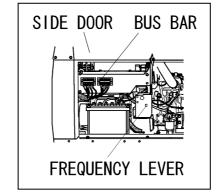
Turn the selector switch and the metal bus bars to the other frequency as per the drawing.
